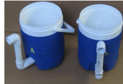
Figure 1. Leachate collection vessels built with a 2-gallon (7.57L) insulated plastic water cooler. Photo credit: Phytosphere Research.
