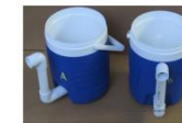
Figure 1. Leachate collection vessels built with a 2 gallon (7.57L) insulated plastic water cooler. Photo credit: Phytophthora Research.
